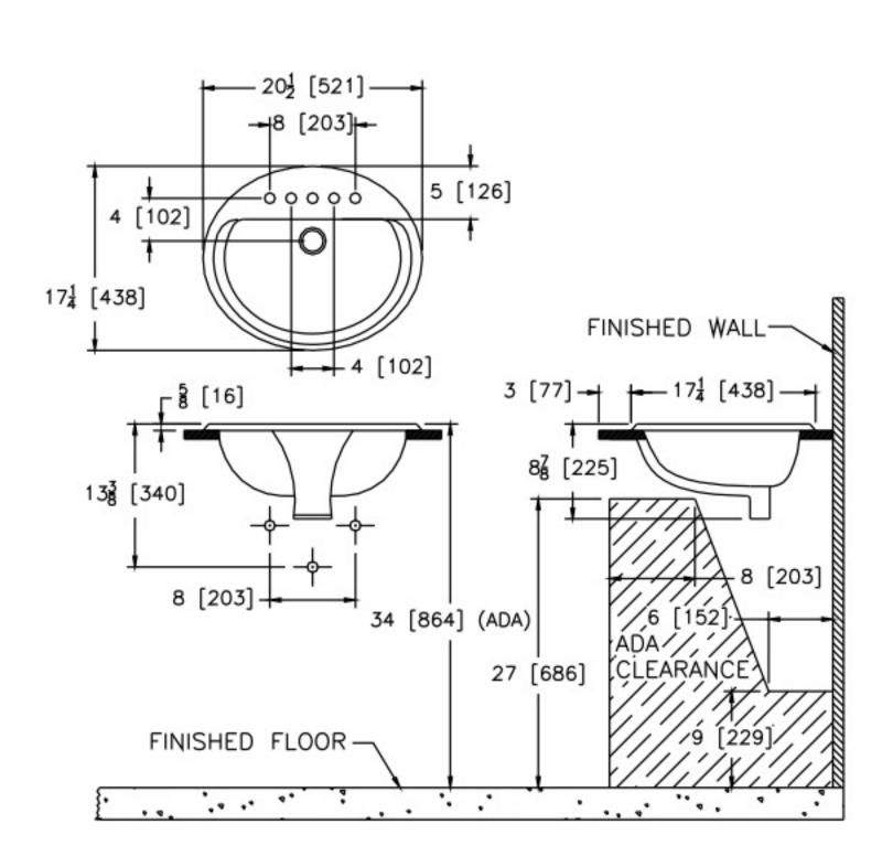
These dimensions and specifications are subject to change without notice. Fixture dimensions meet ANSI/ASME standard A112.19.2 and CAN/CSA B45 requirements.
